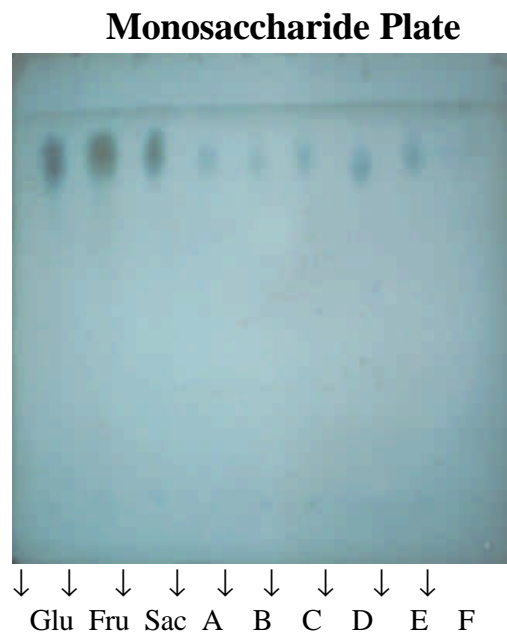
Figure 2. Thin Layer Chromatography of Cassava Samples and Standards.
